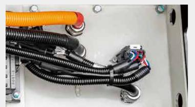
The power plug is fixed on the truck body to avoid damage from battery installment.
