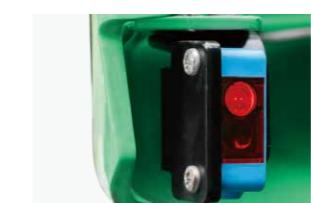
Foot detection sensor - trucks slows down or stops if operator's foot is detected outside of the platform contours (Option).
