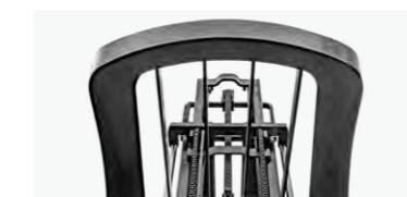
The truck with assembly overhead guard can protect the driver's safety in case of high-position cargo falling.
