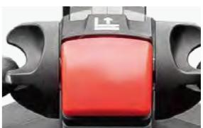
The emergency button on the tiller head can effectively avoid the harm to the driver.
